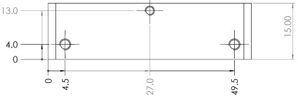
Break angles with chamfer 0.3 to 0.5 x 45°
