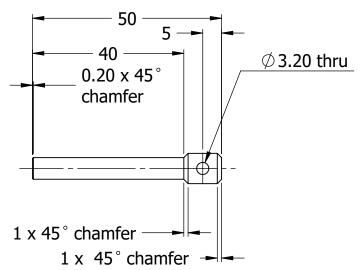
GENERAL TOL. UNLESS SPECIFIED ISO 286-2 1988 MACHINING JS13 FABRICATION JS 16 REMOVE ALL BURRS & SHARP EDGES DO NOT SCALE DRAWING. SCALE: 1:1 FINISH: Non
