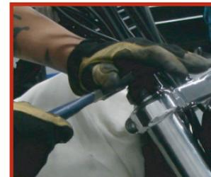
5. Adjust the RSD fork cap using a 5/16" hex wrench to the desired preload setting. Rotating the adjuster clockwise will increase fork preload from the initial setting.
